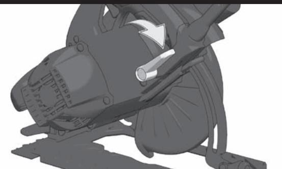
Adjust the cutting depth to the thickness of the workpiece. Less than a full tooth of the blade teeth should be visible below the workpiece.
